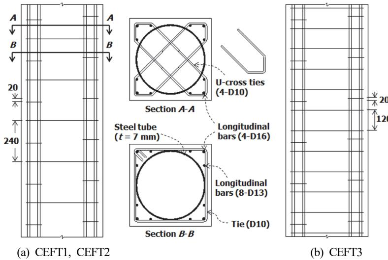
Fig. 2. Reinforcing details of CEFT columns
