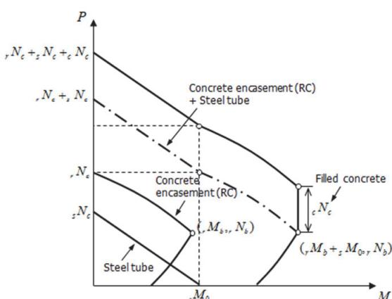
Fig. 10. Axial load-moment relationship of AIJ SRC provision<sup>[9]</sup>
