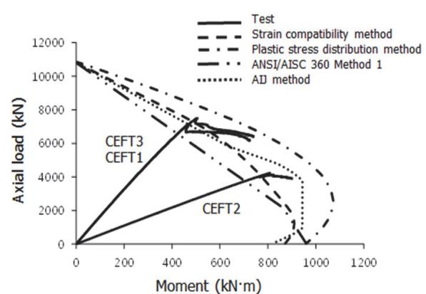
Fig. 11. Axial load-moment relationships of CEFT columns
