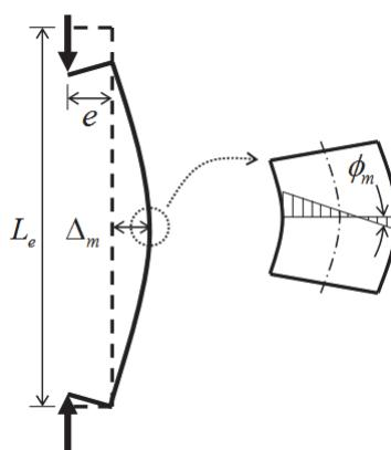
Fig. 8. Deformed shape for sectional analysis
