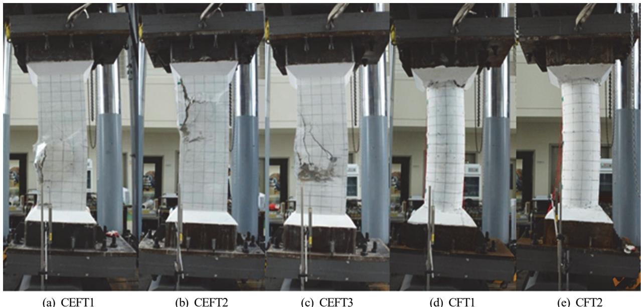
**Fig. 4. Failure modes at the end of the test**
