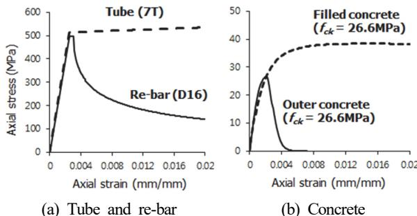
Fig. 7. Uniaxial compressive stress-strain relationships for fiber analysis
