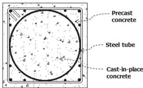
**Fig. 1.** Cross section of circular CEFT column
