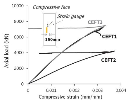
Fig. 6. Strain distribution
