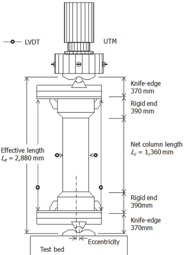
Fig. 3. Test setup for eccentrically loaded specimens
