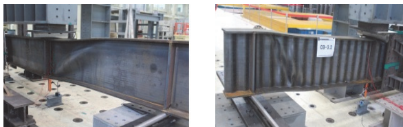
(b) CP-3.2 failure shape of specimen
