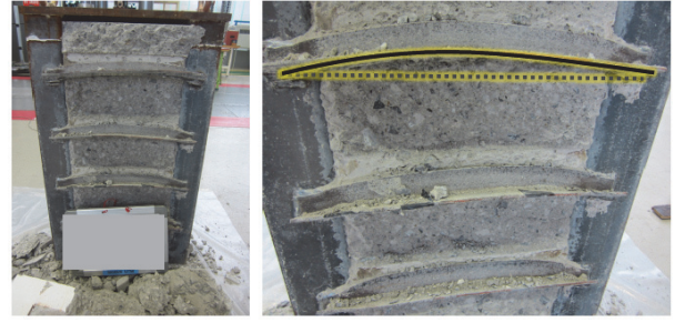
Fig. 3. Deformed shape of BESTOBEAM shear connector
