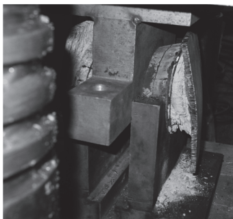
Fig. 7. Weld rupture of end plate for short specimen by Xiao et al. [7]
