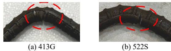
Fig. 3. Representative fracture appearances after rebending
