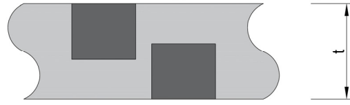
Fig. 10. Location for test specimens with 30mm or more
