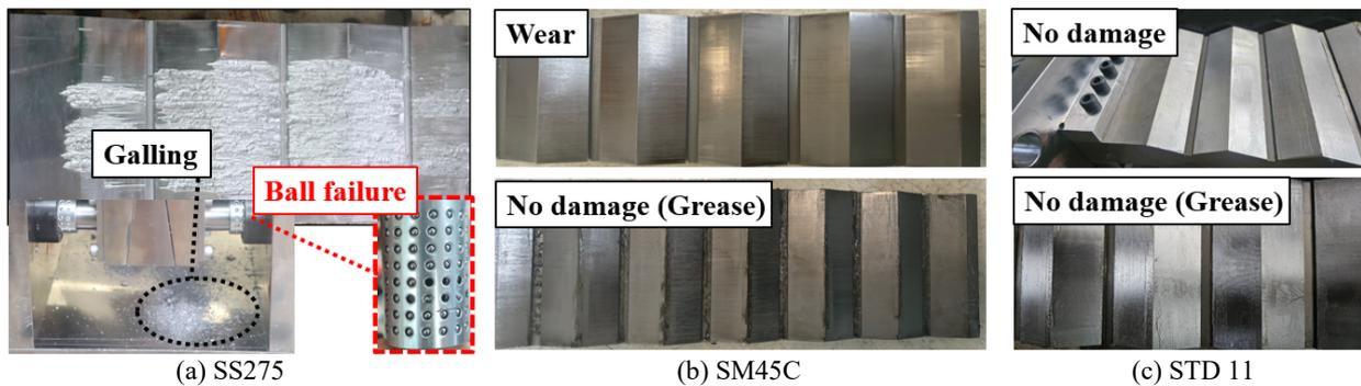
Fig. 12. Friction surface damage
