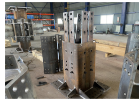
(a) Assemble the inner plate with the lower column
