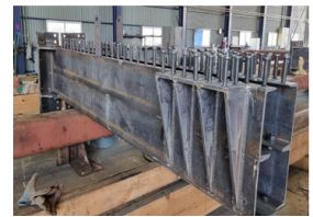
(b) Weld KG beam and endplate
