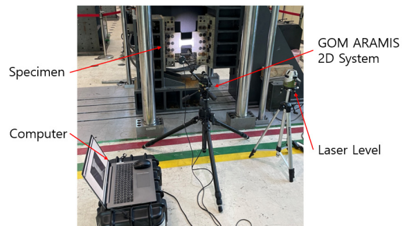
Fig. 8. Camera setup for DIC
