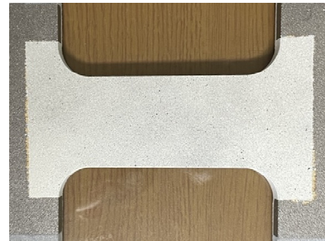
Fig. 3. Specimen of spray speckle pattern
