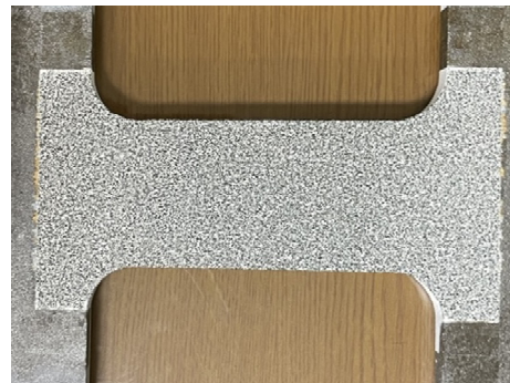
Fig. 4. Specimen of film-free speckle pattern
