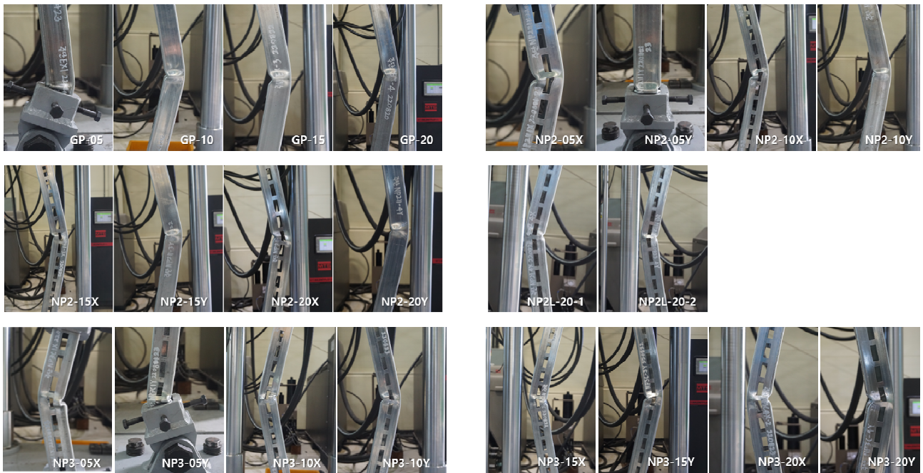
Fig. 5. Failure modes of specimens
