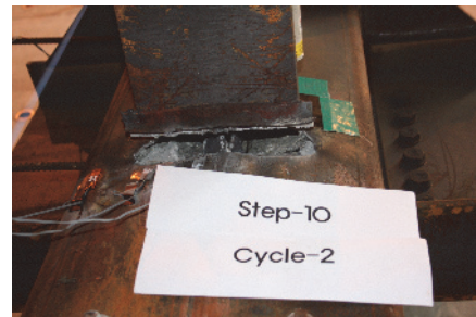
Fig. 12. HBC-2 (failure at lower steel tube during 0.06rad)
