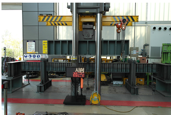
Fig. 5. Overall view of test setup and 3-point loading condition
