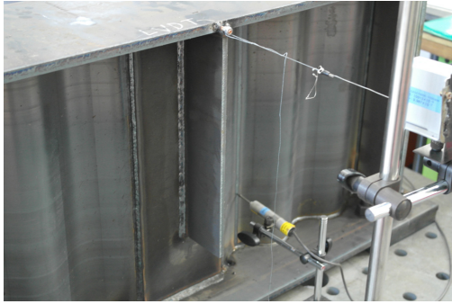
Fig. 9. Lateral displacement measurements of specimen girder
