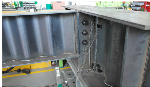
(a) End rotation of the small beam that comprised the FF-E specimen at ultimate load
