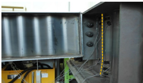
(a) Bending deformation of the reinforcing plate observed in the FP-C specimen girder
