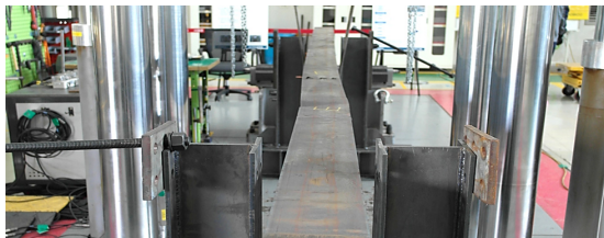
Fig. 10. Lateral torsional buckling observed in LTB-333-2000
