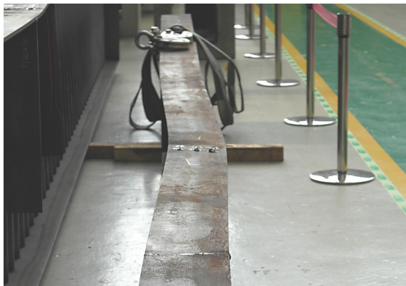
Fig. 13. Permanent deformation of LTB-500-3000
