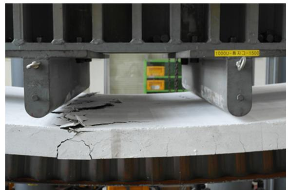
(b) Concrete crushing at loading region
