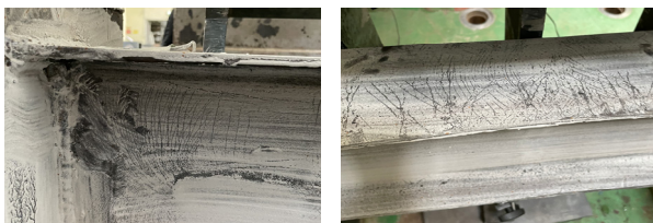
Fig. 15. Fracture mode of beam-PC slab
