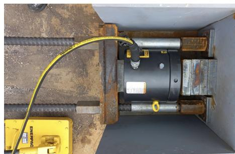
(b) Hydraulic jack and steel rod setting of mock-up specimen
