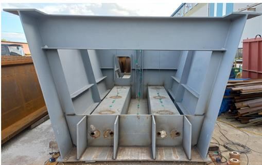
Fig. 6. Mock-up specimen of CTF-steel box girder
