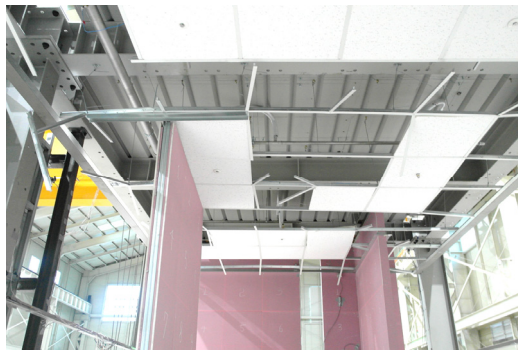
(c) Fallen ceiling area observed at end of tests
