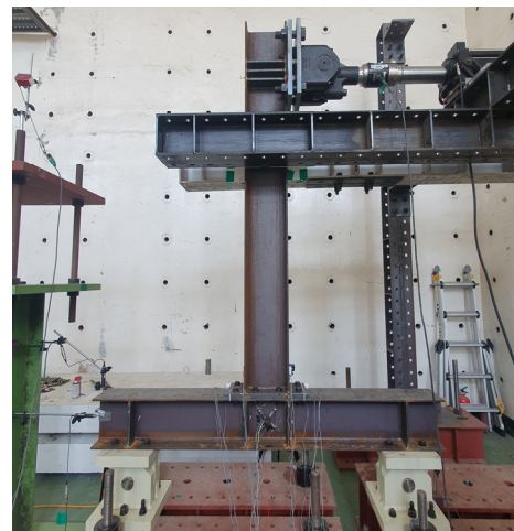
Fig. 6. Set-up for specimen PY
