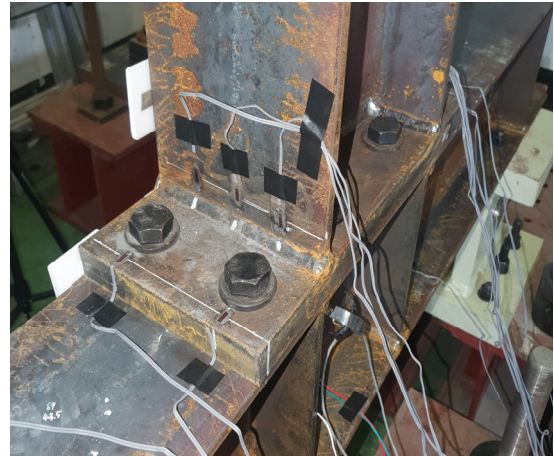
Fig. 15. Detail of attaching strain gauge
