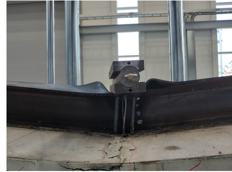
(b) Local buckling near the load point
