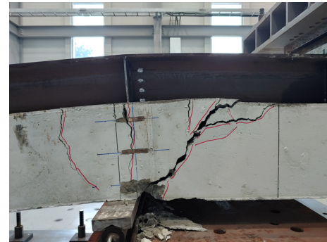
(d) Crack near support point
