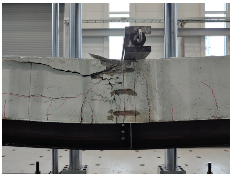
(b) Crack near the load point
