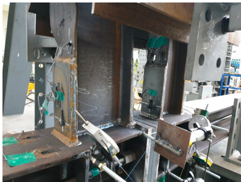
Fig. 7. Failure mode of EX-S-175PT at 8 %
