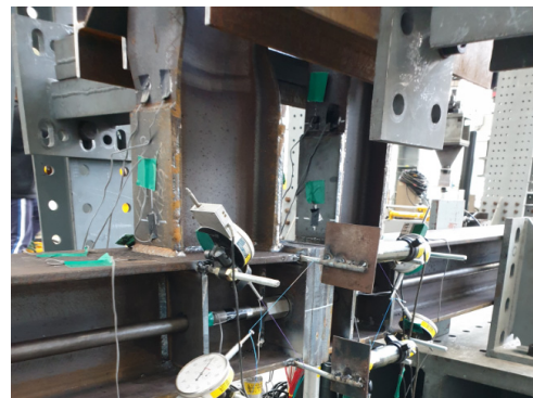
Fig. 9. Failure mode of EX-S-260PT at 7 %
