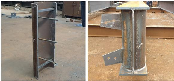
Fig. 2. Plate girder with CFHPS
