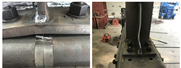
Fig. 13. Test specimen IP14-D32(F) at the end of the test
