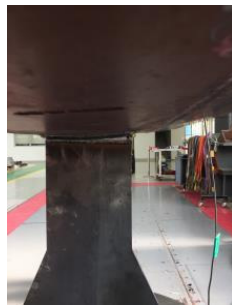
(f) T5 (weld fracture)
