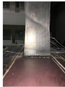
(g) T6 (necking at beam flange)
