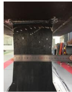
(h) T7 (necking at beam flange)
