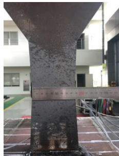
(j) B2 (necking at beam flange)
