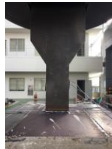
(k) B3 (necking at beam flange)
