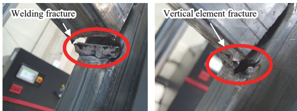
(a) LW1.6 (b) LW2.0 Fig. 24. Ultimate state of line welding
