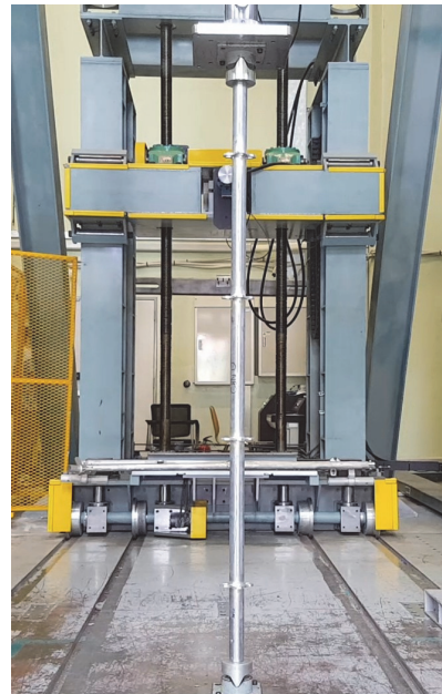
Fig. 5. Test set-up for unit vertical member
