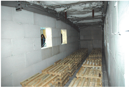
Fig. 8. Wooden cribs used for the fire load
