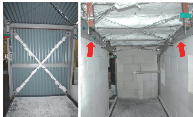
(a) Wall brace (b) Wall and ceiling
