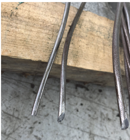
Fig. 6. Configuration of fractured wires of the tensile test using anchor type gripping device
