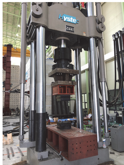
Fig. 3. Photograph of 5,000 kN UTM and installed anchor type gripping device
