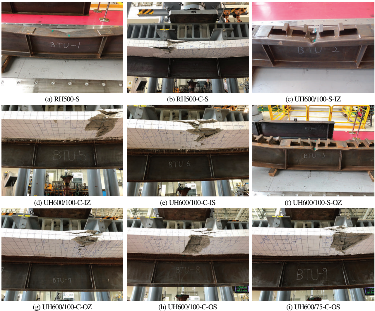
Fig. 5. Failure modes of test specimens
