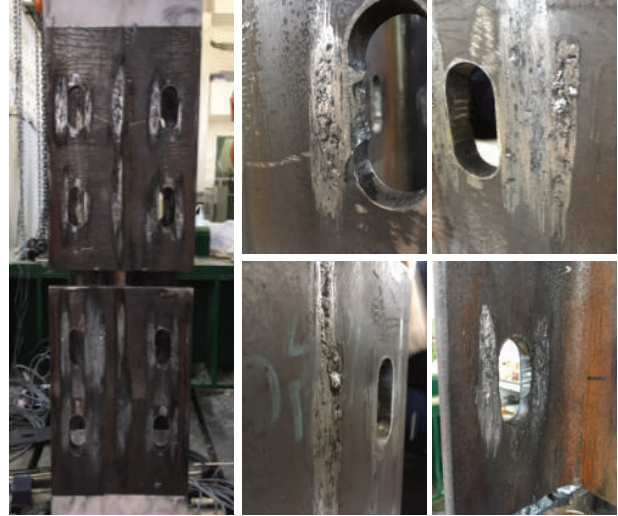
Fig. 17. Friction surface damage due to repetitive force
