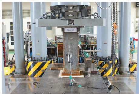
Fig. 4. Installation view of CFT-Column specimens
