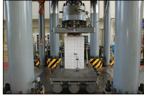
Fig. 2. Installation view of Push-out specimens
