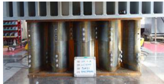
(a) Bolt failure
