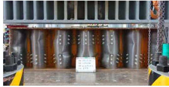
(a) Local buckling failure
