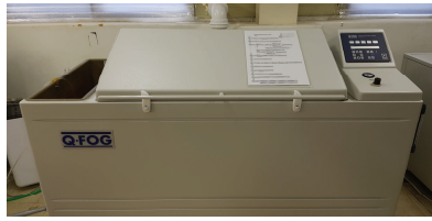
(a) Salt spray acceleration test
