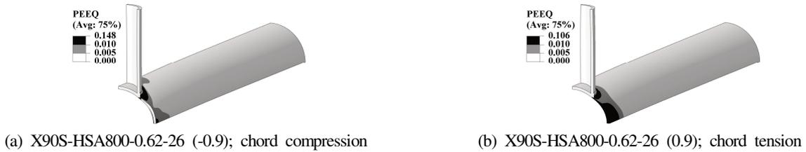
Fig. 10. Equivalent plastic strain distribution of pre-stressed joints at 3% out-of-plane deformation
