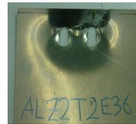
(c) Curling+Tensile crack (ALZ2T2E36)
