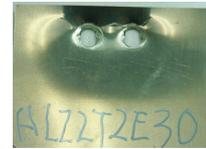
(b) Curling+Tensile crack (ALZ2T2E30)
