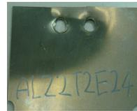
(a) Shear fracture (ALZ2T2E24)
