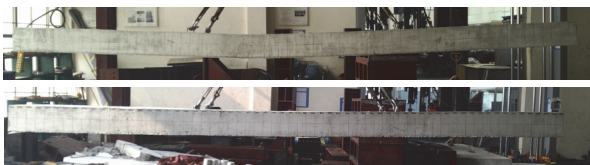
Fig. 16. Failure Shape of experiments for bending test
