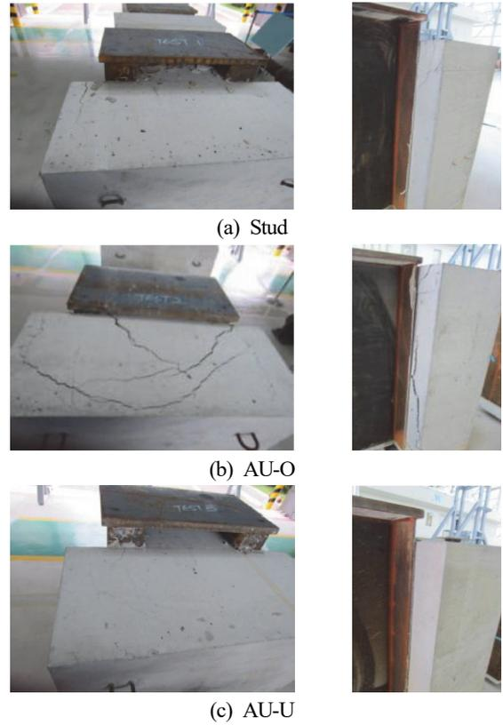
Fig. 9. Failure mode of specimens (continuous type)
