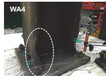
(c) Local buckling at beam flange section
