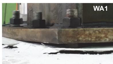
(b) Pull-out failure of concrete
