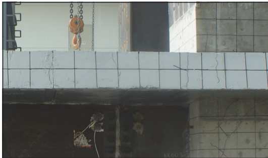
(b) slab section
