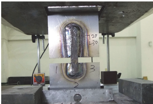
Fig. 5. Set-up of specimen and transducers (LVDTs)
