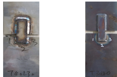
(b) Arc welding (FT40L30-A) (c) TIG welding (FT30L40-T)
