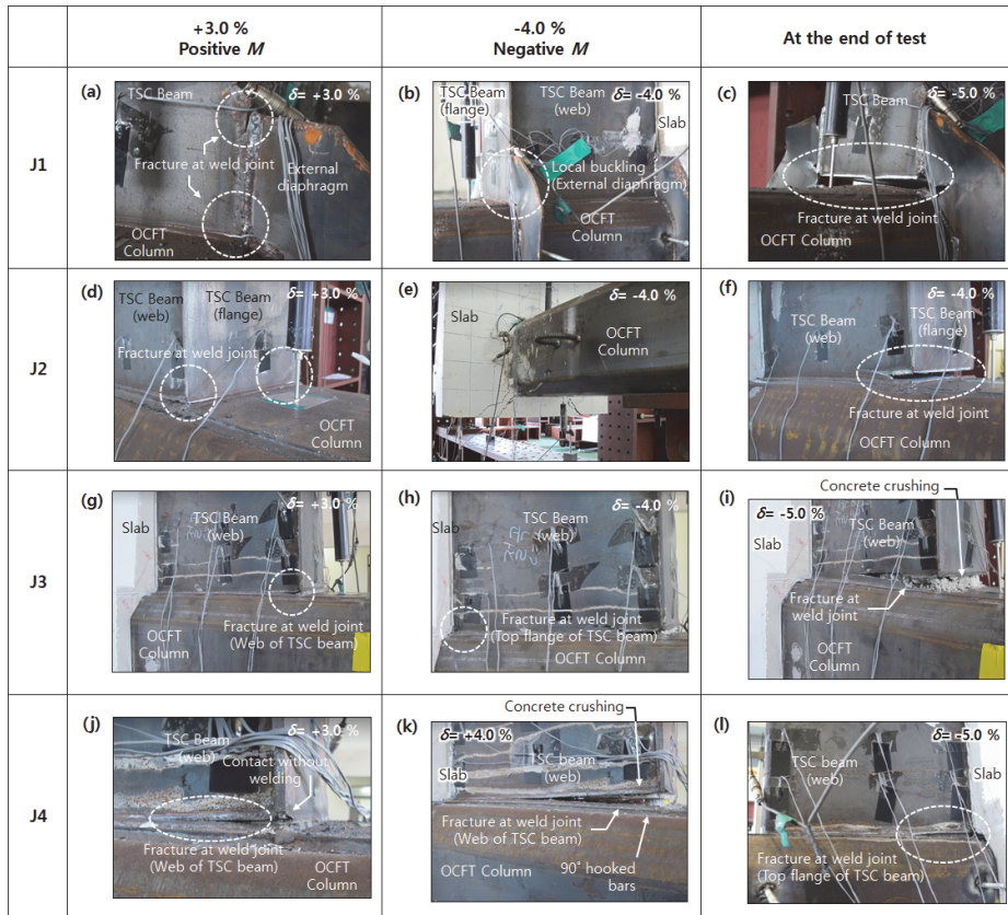
Fig. 6. Failure mode at beam-to-column connection
