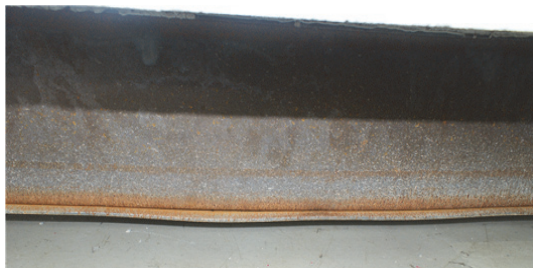
Fig. 14. After test, bottom plate of S3-F3T6-R
