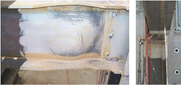
Fig. 8. LB and LTB of WEAK-DB700-SW at 4% story drift
