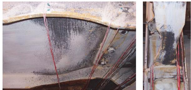
Fig. 11. LB and LTB of WEAK-DB600-SW at 5% story drift
