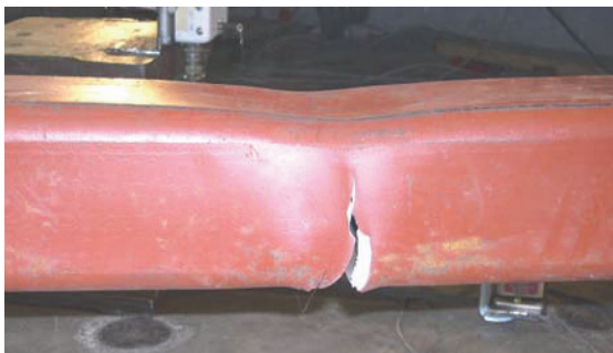
(c) HSS5: Brace fracture (37Cycle, -3.26% Drift)
