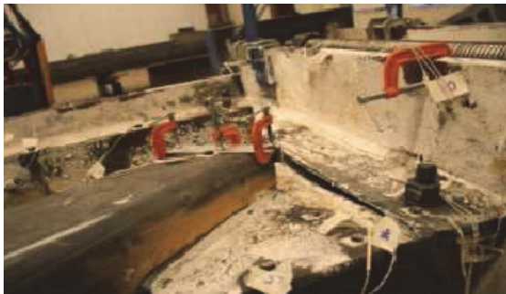
(a) NCBF3: Weld fracture of gusset-to-shear tab (24Cycle, -1.63 Drift)
