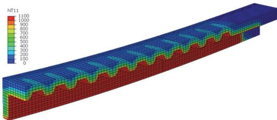
Fig. 13. Example of numerical simulation result of the partially encased beam (HB-PE-L3, 1/4 model)
