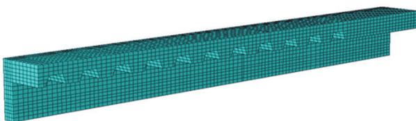
Fig. 10. Finite element model for the thermal-stress analysis (HB-PE-L3, 1/4 model)
