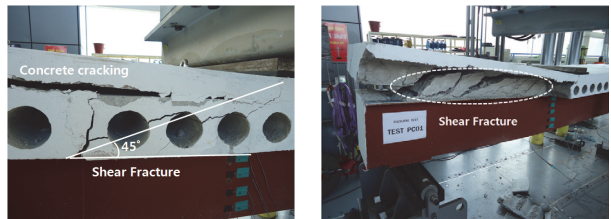
(b) Failure mode(PC01)
