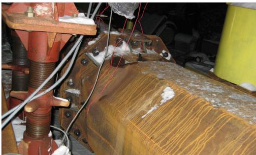
Fig. 6. Deformed shape after load peak
