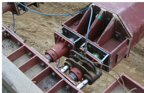
Fig. 3. End connection element
