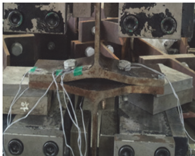
(b) Type of bolt and flange fracture
