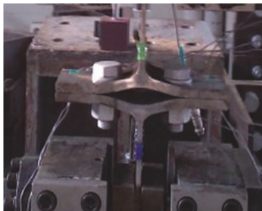
(c) Type of flange fracture
