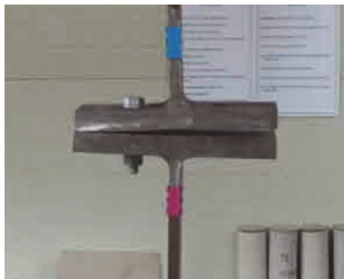
(a) Type of bolt fracture
