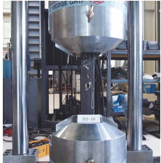
Fig. 2. Tensile test for plate with bolt hole
