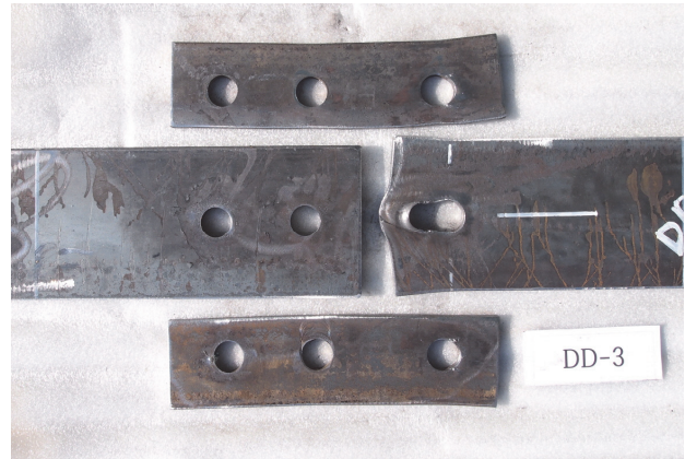
Fig. 6. Configuration of bearing failure
