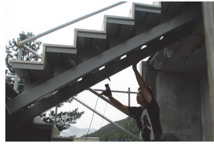
Fig. 8. Impact hammer test
