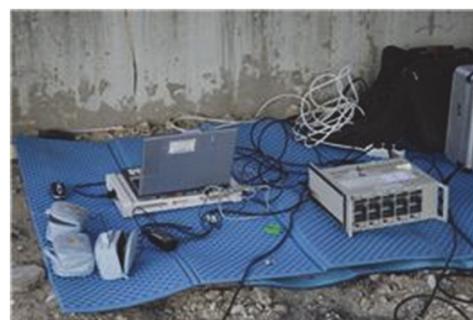
Fig. 4. Vibration measurement system [7]
